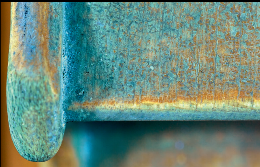
Figure 5: crequelure and surface texture are still visible on the back of the “Kreisler” (above). Craquelure can also develop as a result of polishing (detail of the C-bout rib on the “Kreisler”, bottom left), a process that drove dirt and rosin to impregnate the open pores of maple “Baron Knoop” (bottom right).
